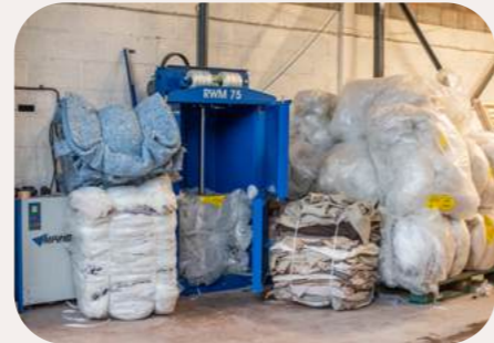
Our baling machine with bales of offcut recycled denim, fabric and plastic packaging.
